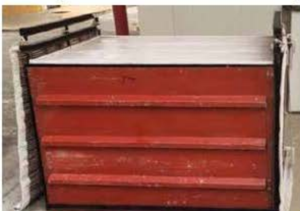
Livestock housing module for winter season with opaque panel
