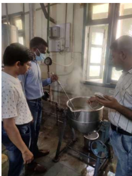
Ghee preparation using modified pre-stratification method with lesser energy requirement at Dairy Engineering division
