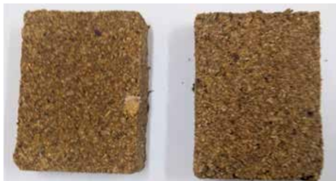
Multi-ingredients blocks prepared with the byproducts available after production of fatty acid methyl ester from non-edible oils
